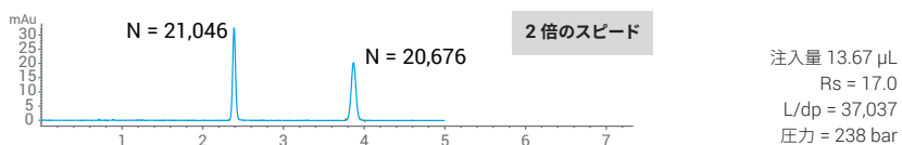
InfinityLab Poroshell 120 EC-C18, 4.6 x 100 mm (L1), 2.7 μm
