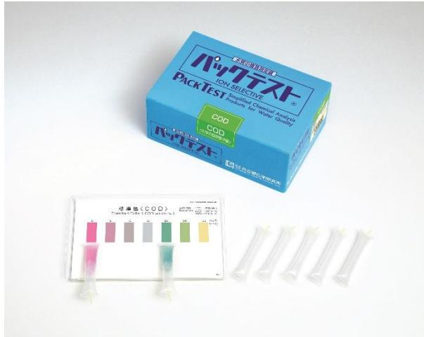
PACKTEST is the most simplified analysis instrument for water quality check. You can easily examine the water quality by sucking the water sample up into a tube containing reagents and comparing its color with the Standard color after the reaction time. It is ideal for controlling the quality of water, such as groundwater, river water, industrial water, wastewater from factory, and more.
