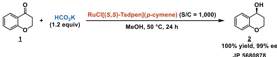
To a solution of ketone **1** (1.48 g, 10 mmol) in MeOH (6 mL) was added potassium formate (1.0 g, 12 mmol) and **Ru catalyst** (6.4 mg, 0.01 mmol) under argon atmosphere. After stirring for 24 h at 50 °C, the reaction was completed (100% conversion) and the solution was cooled down and diluted with H<sub>2</sub>O. The solution was extracted with EtOAc, and the combined organic solvent was concentrated to afford alcohol **2** (99% ee).
